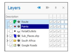
The way the tool works is that the bottom layer is always taken as the baseline of comparison and will be the layer whose geometries will be included in the new joined layer created. In this case it is my **Points** layer. The tool will do a join based on how far the route is from each point.
